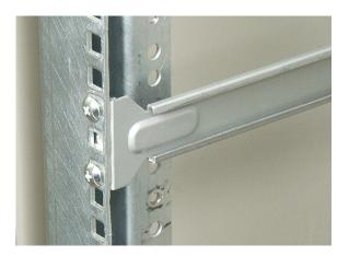
**8** With the front of the server facing you, lift the server and insert it into the cabinet from the front, then position the disk guides so they fit into the cabinet rails. (Your server may be different than the server shown in the example.)
